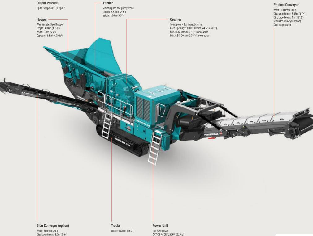
CAT C9 ACERT 242kW (325hp) Tier 4F / Stage 4: Scania DC9 385A 257kW (350hp) Fuel tank capacity: 500 L (132 US Gal)
